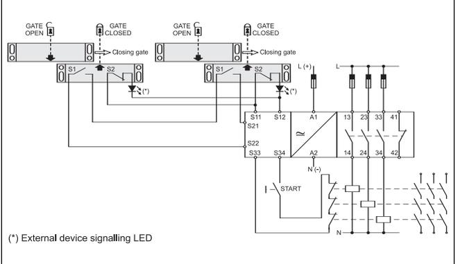
**NSC02D - Mechanical switch and one access monitoring (Single channel)**
