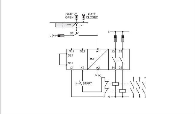
**NSC13D - Mechanical switch and one access monitoring (Single channel)**
