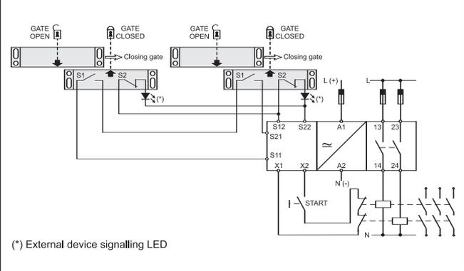
**NSC13D - Magnetic sensors and two accesses monitoring (Double channel)**
