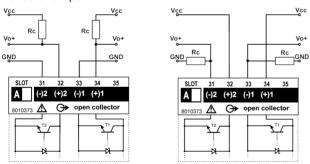
The grounds of the outputs are separated, and therefore it's possible to carry out, for the same module, two different connections. The load resistance (Rc) must be designed so that the closed contact current is lower than 100mA; the VDC voltage must be lower than or equal to 30V.
