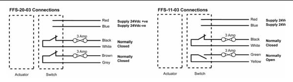
Contact configurations show under closed condition for guard device.
