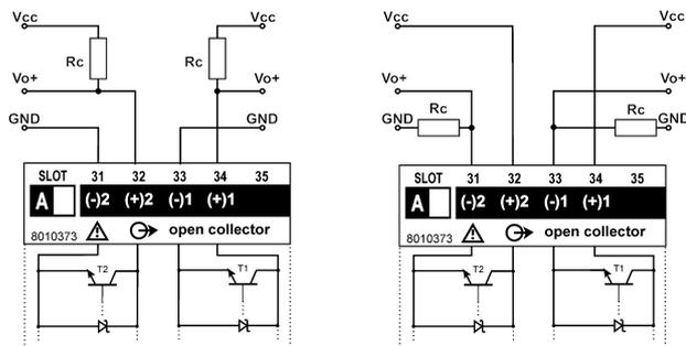
The grounds of the outputs are separated, and therefore it's possible to carry out, for the same module, two different connections. The load resistance ( $R_c$ ) must be designed so that the closed contact current is lower than 100mA; the VDC voltage must be lower than or equal to 30V.
