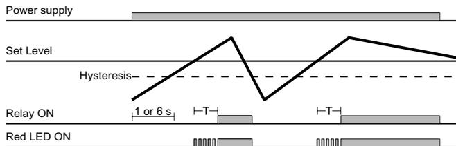
**Under voltage - Latch function - N.D. relay**
