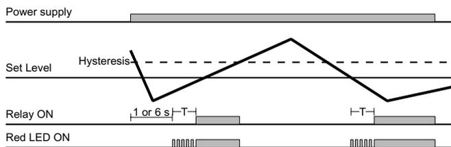
**Over voltage - Inhibit function - N.D. relay**
